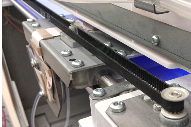
Figure 1: Belt and pulley configuration of x-y gantry 9
